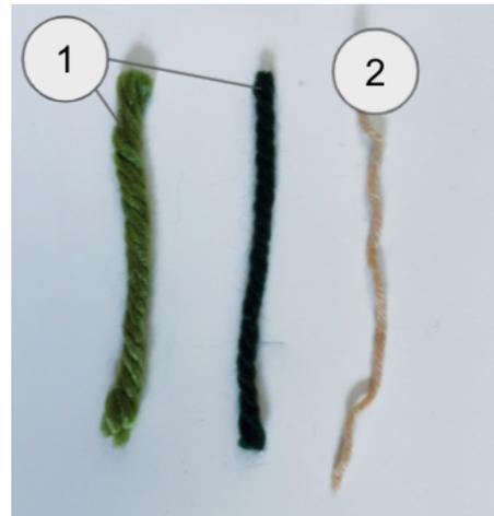
**Figure 4: Normal yarns we have access to: 1. 100% acrylic chunky yarn. 2. 100% acrylic thin yarn.**
